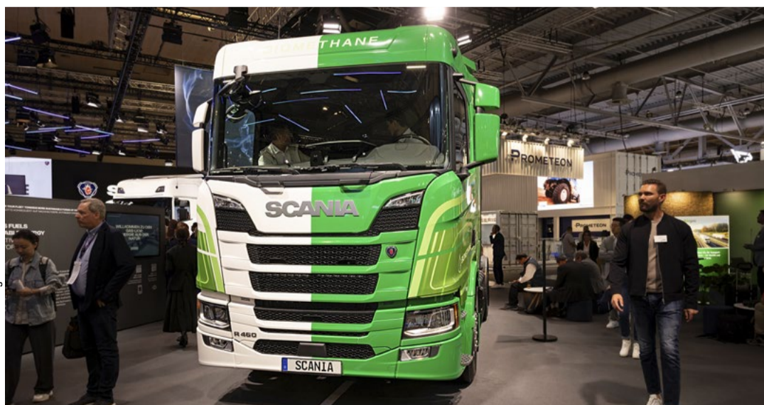
The two-tone Scania R 460 with gas engine can be supplied with both compressed biogas (CBG) and liquefied biogas (LBG). This means it can refuel at any gas filling station and reduce CO 2 emissions by up to 90 percent, according to the manufacturer.
